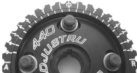
Notice how the “ 0 “ line on the outer lines up with the “ 0 “ line on the **inner** and the bolts are centered in the slots. Also note that the further most lines on the **inner** are both under the 9° mark in both the Advanced and Retard section. This helps in finding true 0°.
